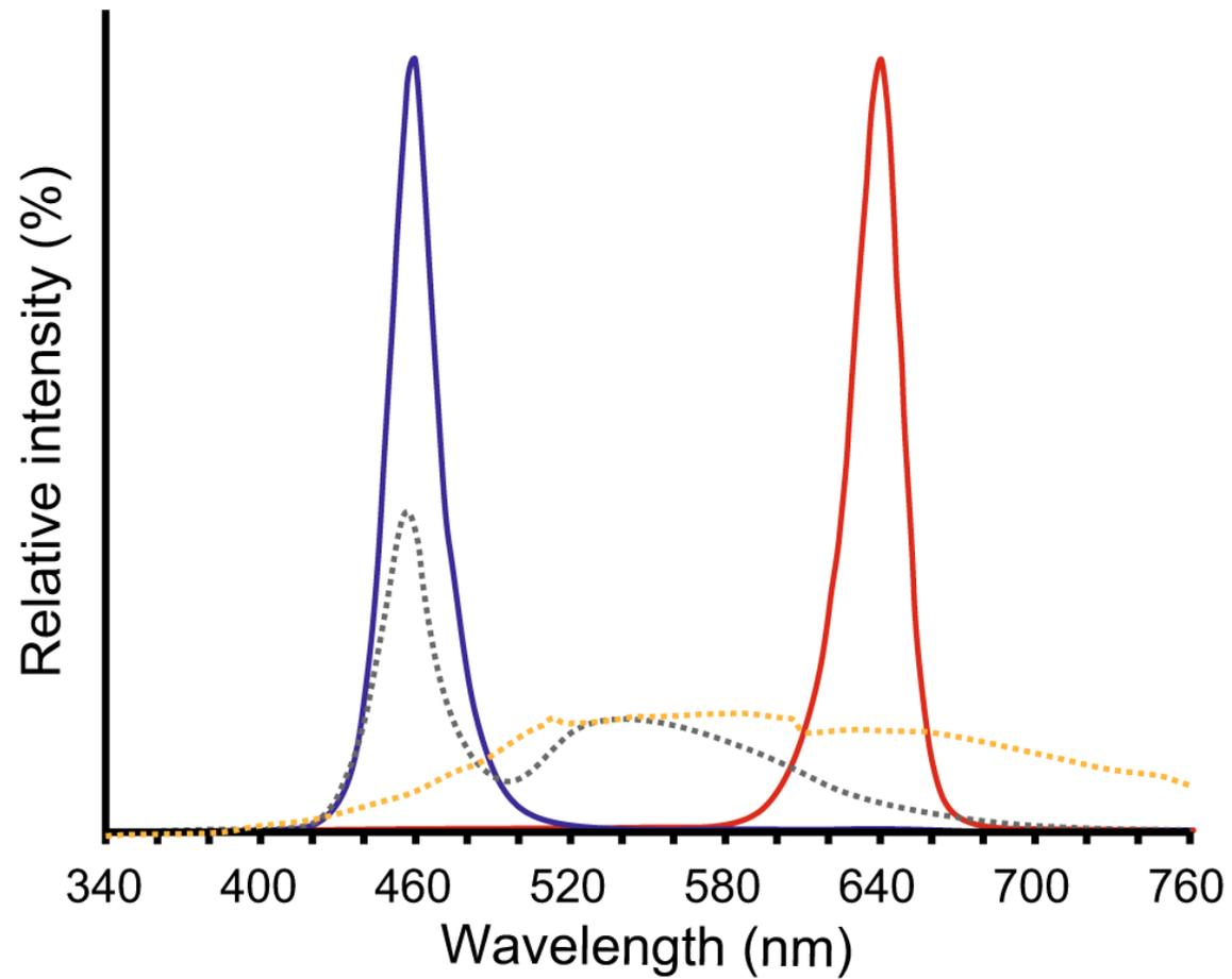
**Fig. 1** Light spectra of LED light sources. Light spectra of *white* light (*black dashed line*), *blue* light (*black line*), *red* (*gray line*), and halogen light (*gray dashed line*) are shown. The total areas of light intensity in the wavelengths of the photosynthetic photon flux density (400–700 nm) were equalized
